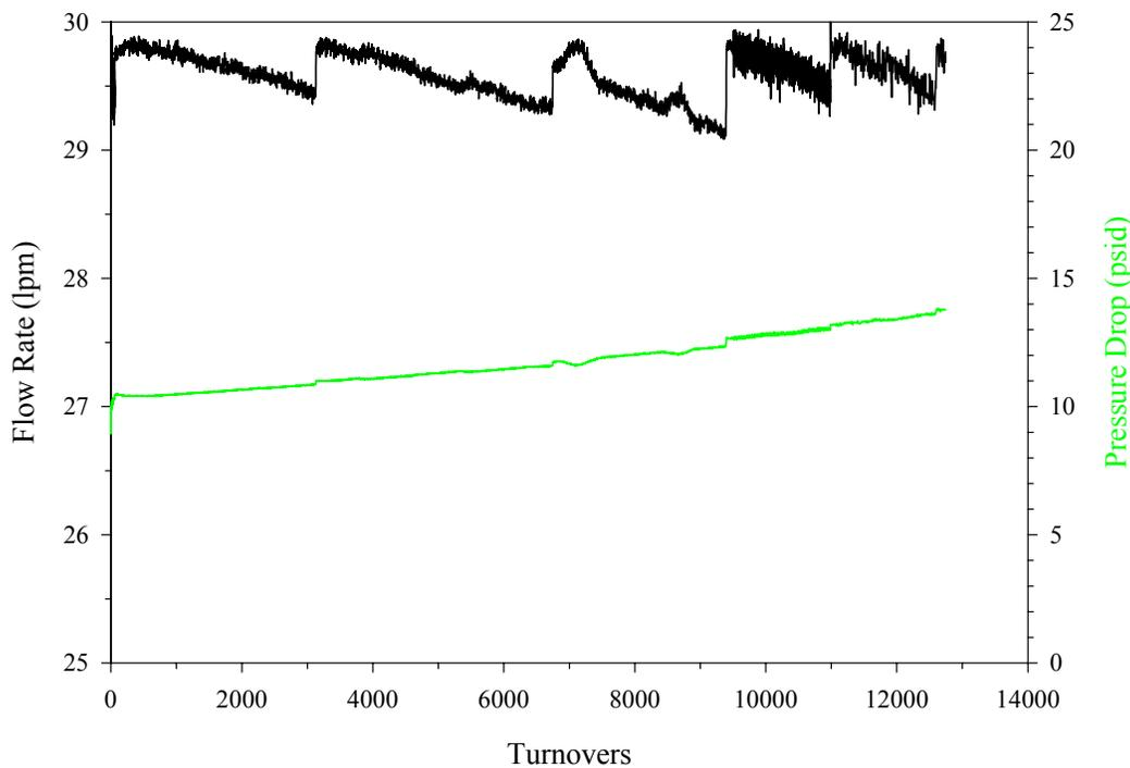
The  $\Delta P$  measured across each CMP3 filter during the beginning of each test are shown in Figures A4-A6 for the ASTI, Yamada, and Levitronix pumps, respectively. Approximately one turnover was needed to adjust the pumps to the desired flow rate of 29.5 lpm. Once this flow rate was achieved, only minor adjustments in the pump air pressure or speed were required.
