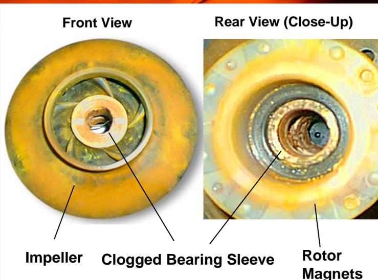
**Figure 2:** Rotor of Mag-Drive pump after 3 weeks operation with gold sulfite with close up of clogged bearing (rear view)
