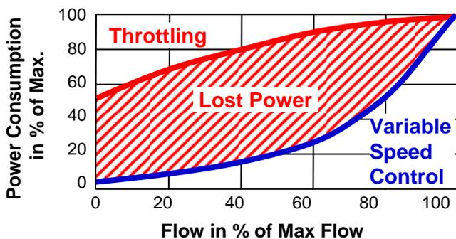
**Figure 7:** Power consumption vs. flow rate for different flow control schemes
