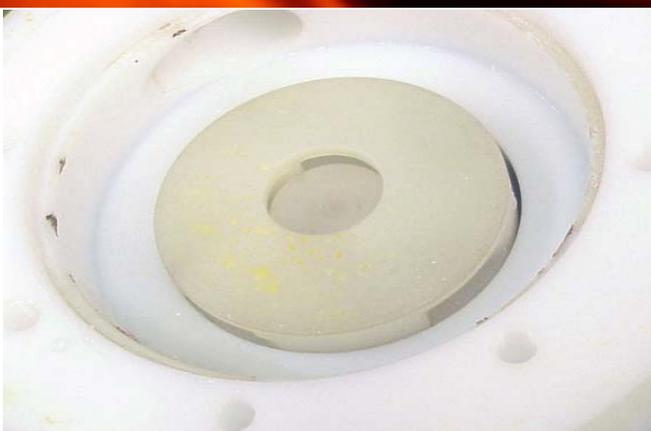
Figure 5: Levitronix pump after 6 month operation with gold sulfite
