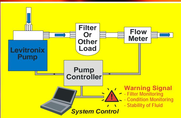
**Figure 8:** Closed-loop flow control with Levitronix Pump
