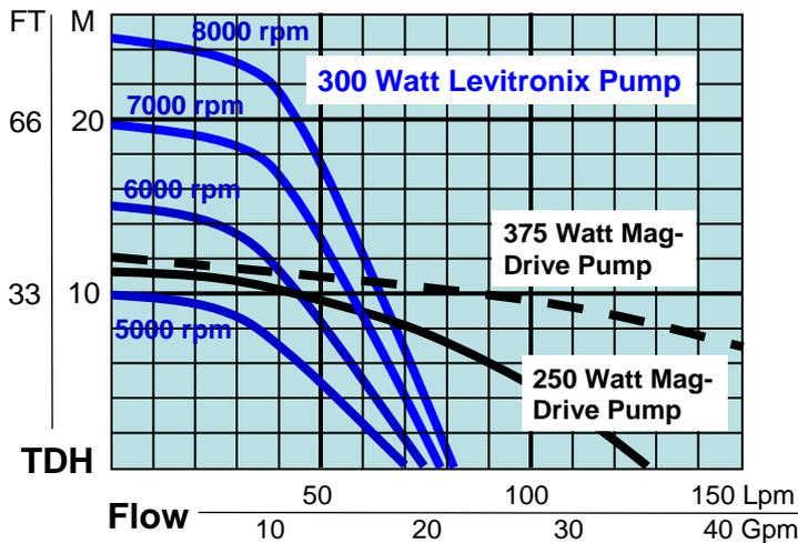
**Figure 6:** Flow/Pressure curves of 300 Watt Levitronix pump compared to typical 250 Watt and 375 Watt Mag-Drive pump
