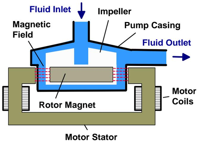
Figure 3: Schematic of bearingless pump
