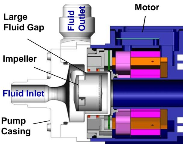
Figure 4: Cross-section of bearingless pump
