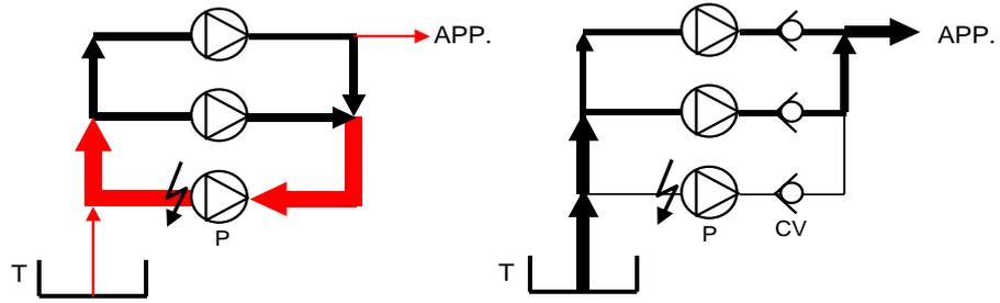
**Figure 2: Pump failure without check valve (left)
