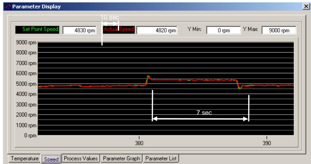
Figure 15: Dynamic adjusted pump speed to maintain defined output pressure of 4 bar.
