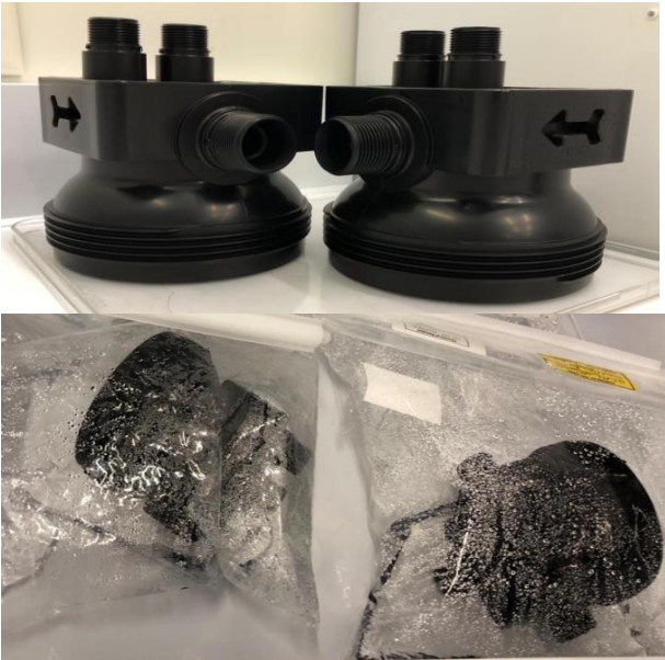
Filter Heads in extraction bags Step = chemical extraction
