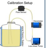
During process operation, the viscometer can be readily integrated into the process stream to measure real-time concentration.
