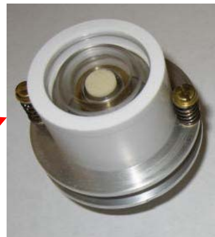
Sample holder with sapphire window and load cell
