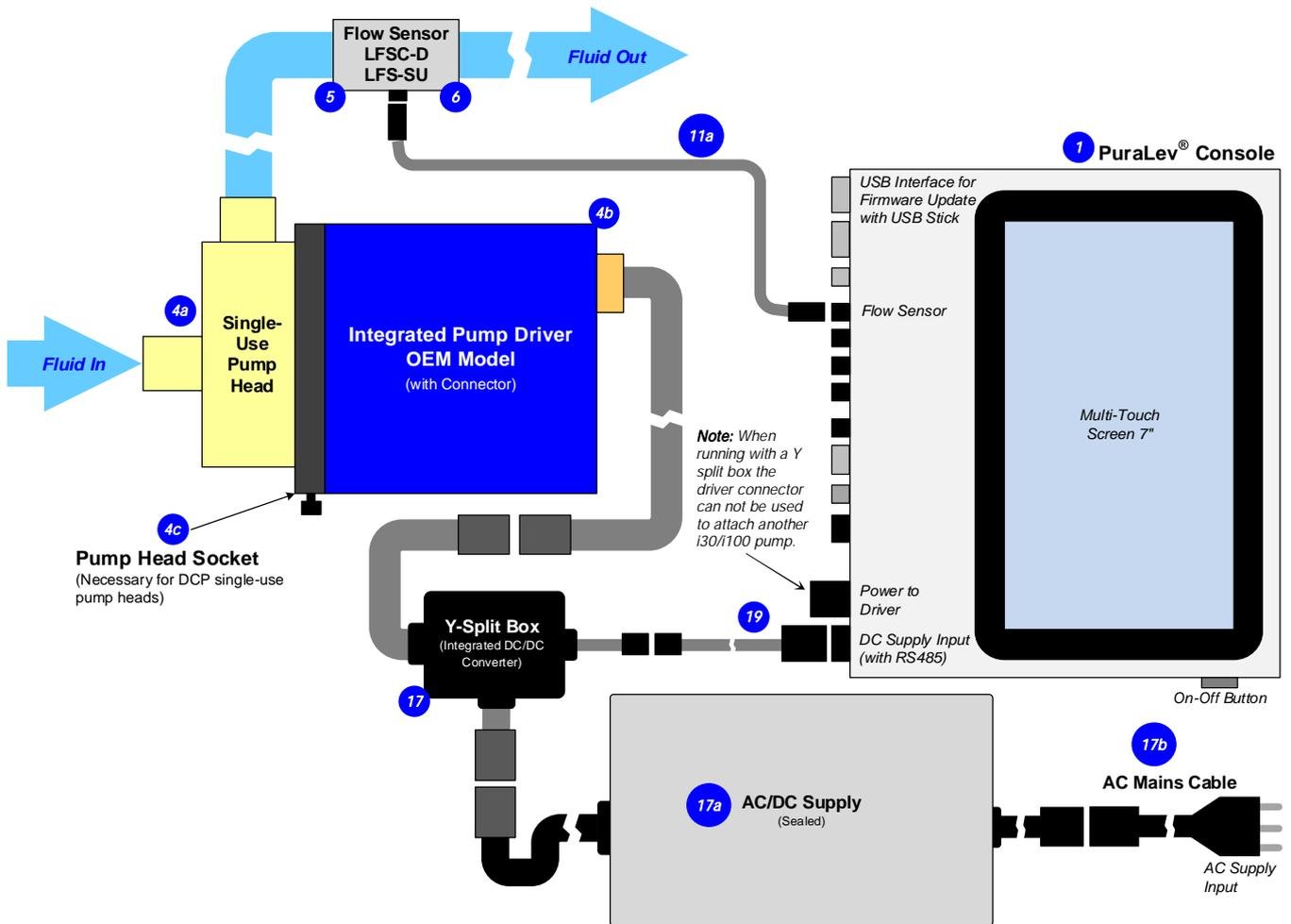
Figure 9: Stand-alone pump system configuration of LCO-i100 console and PuraLev® i600 pump system with flow control or flow monitoring
