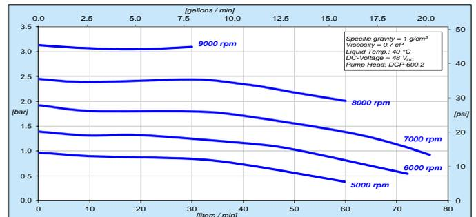
Figure 7: Pressure/flow curves with PuraLev® i600SU (DCP-600.2 pump head)
