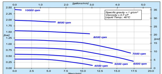
Figure 6: Pressure/flow curves with PuraLev® i100MU (LPP-200.16/17 pump heads)
