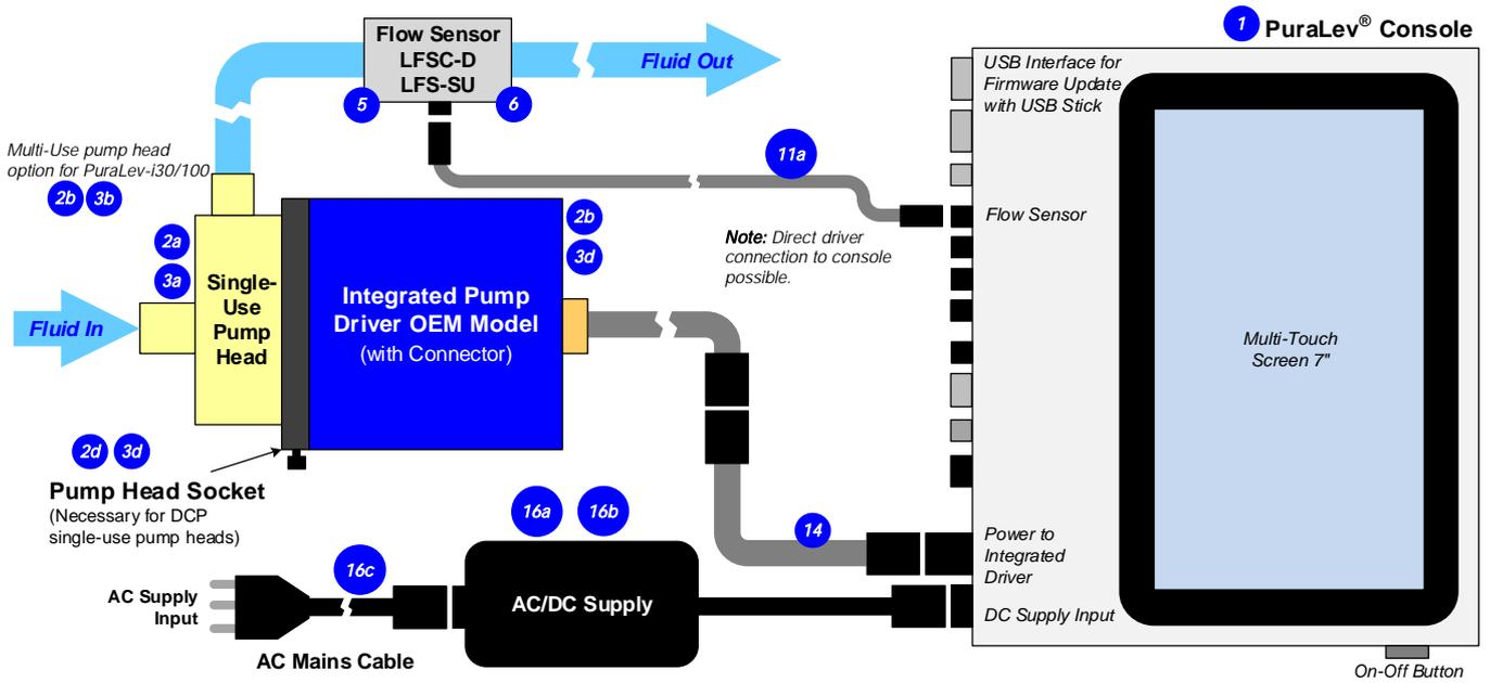
Figure 8: Stand-alone pump system configuration of LCO-i100 console and PuraLev® i30/100 pump systems with flow control or flow monitoring
