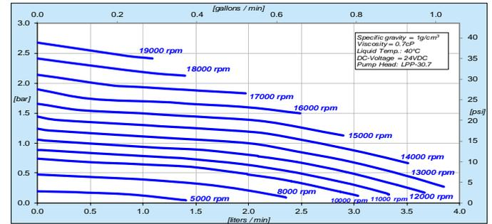
Figure 4: Pressure/flow curves with PuraLev® i30MU (LPP-30.7 pump head)
