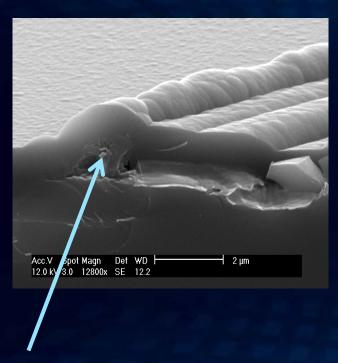
Caused by extensive chemical flow, visible after plasmanitrid deposition
