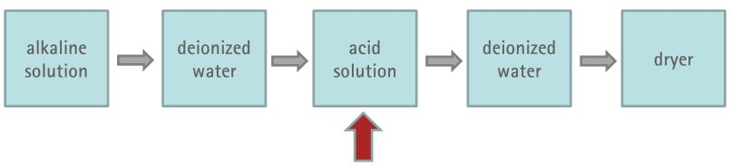
GaAs wafer are sensitive for particle contaminations in acid solutions.
