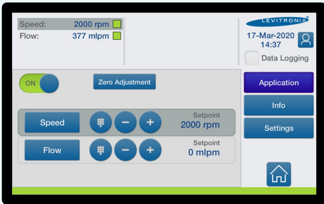
Figure 2: Start-up menu of touch screen
