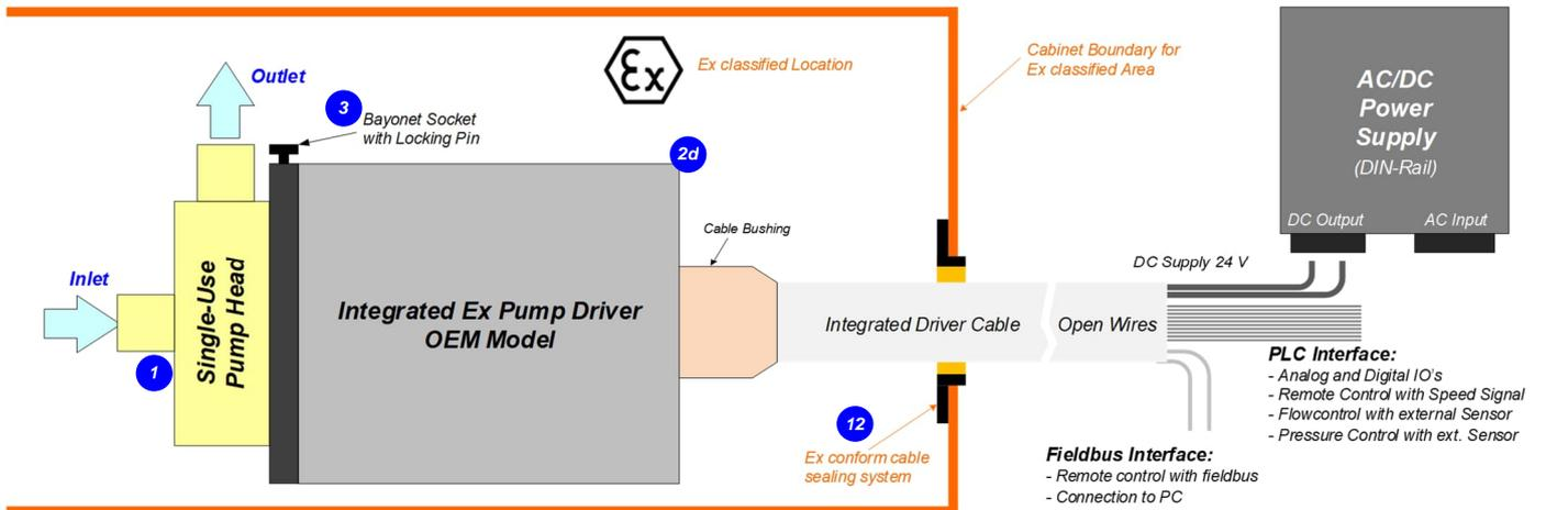
**Figure 8:** ATEX/IECEx "OEM" configuration
