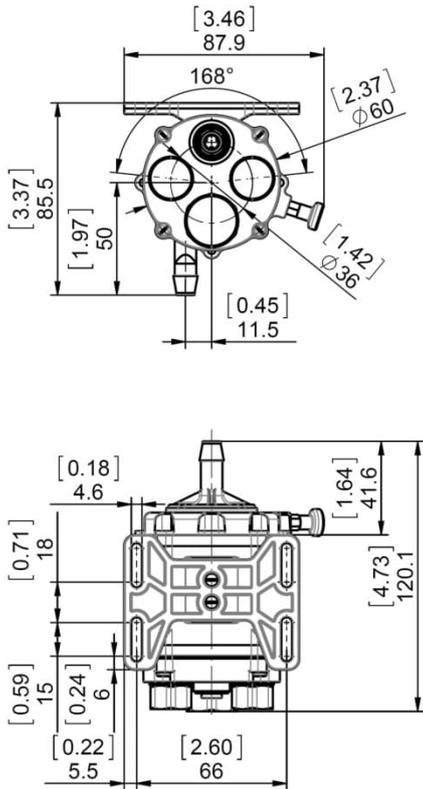
Pump Head Inlet and Outlet Fitting:
