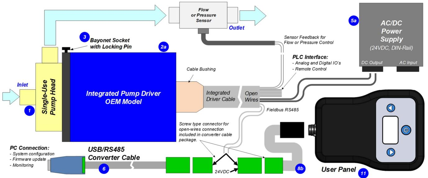
**Figure 7:** Standard "OEM" system configuration
