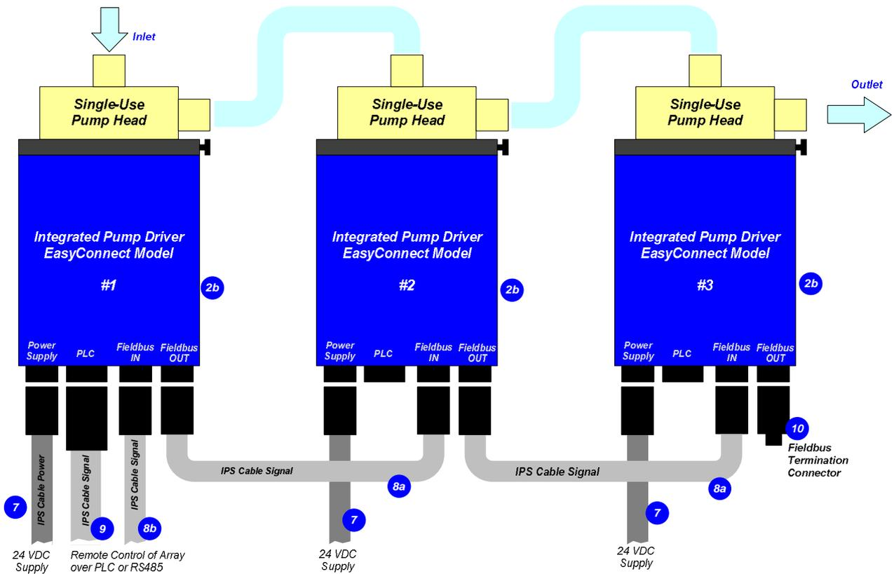
**Figure 10:** Serial pumping configuration with "EasyConnect" models
