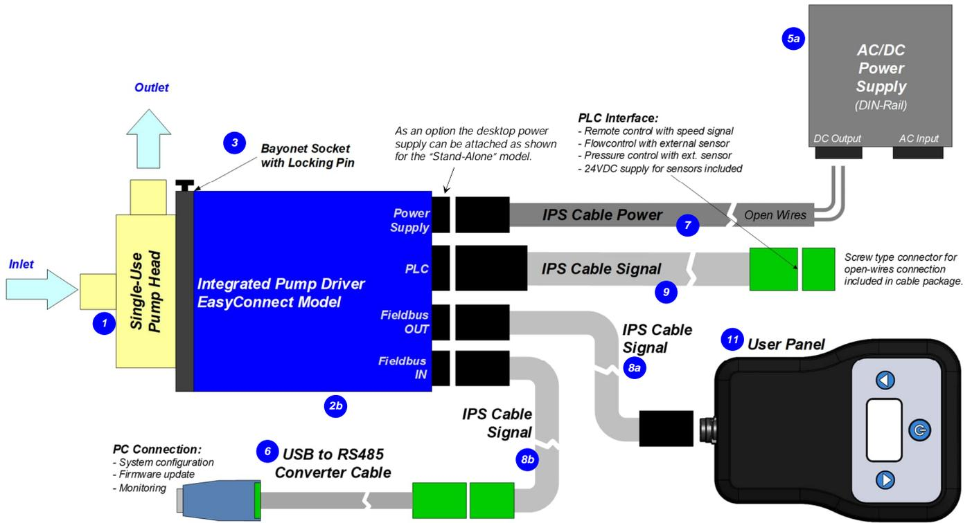
**Figure 9:** Standard "EasyConnect" system configuration with main accessories
