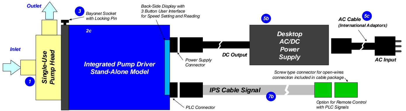
**Figure 6:** Standard "Stand-Alone" system configuration with main accessories
