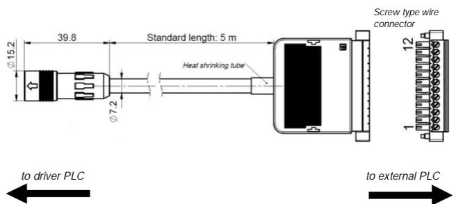
Figure 17: Basic dimensions and specifications of standard cables
