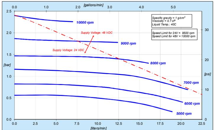
Figure 4: Pressure/flow curves
