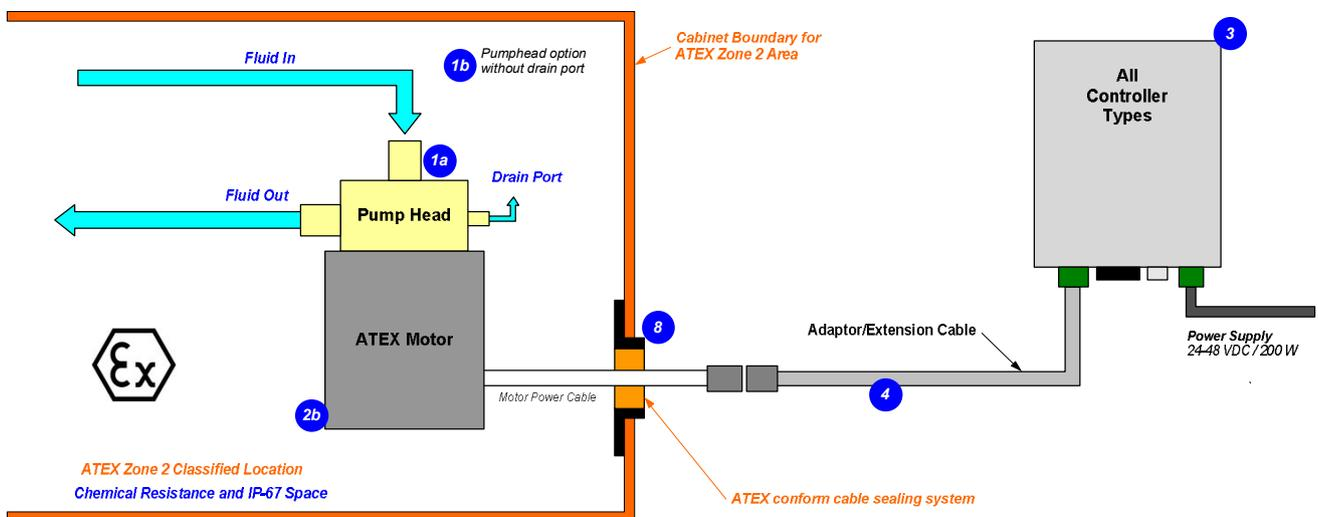
Figure 8: System Configuration for ATEX / IECEx applications
