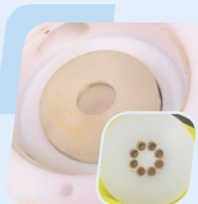
Levitronix® pump after one year of operation with gold sulfite solution
