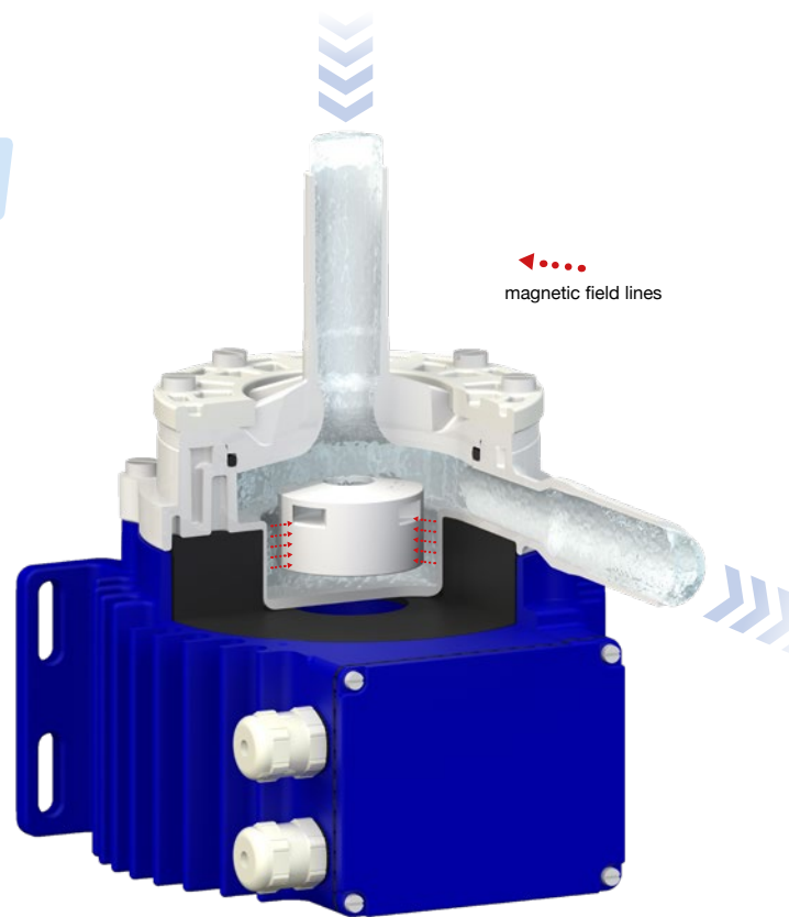
The magnetic levitation allows high rpm resulting in continuous, large flows.
