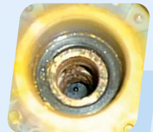
Magdrive pump after one month of operation with gold sulfite solution
