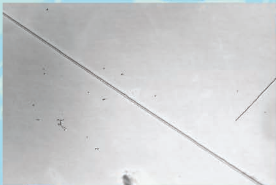
ULK wafer polished with slurry which was recirculated 1000x with a bellows pump
