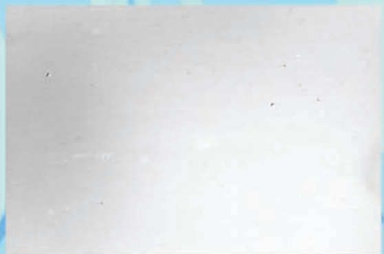
ULK wafer polished with slurry which was recirculated 1000x with a Levitronix pump
