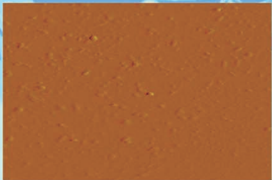
AFM image of wafer surface polished with slurry which was recirculated 1000x with a bellows pump
