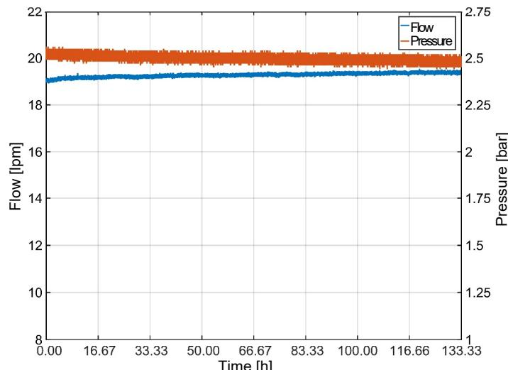
**Flow and pressure 4-piston diaphragm pump**
