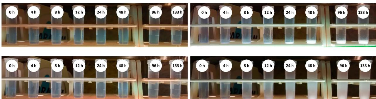
**Figure 4:** Visible turbidity of the lysozyme solution in experiment P1.1/P1.2 at 10 lpm and 1.5 bar with the 4-piston diaphragm pump (right). The upper images show the turbidity in sedimented state and those below, after mixing the samples. The samples of the centrifugal pump show no turbidity or aggregates (pictures on the left).
