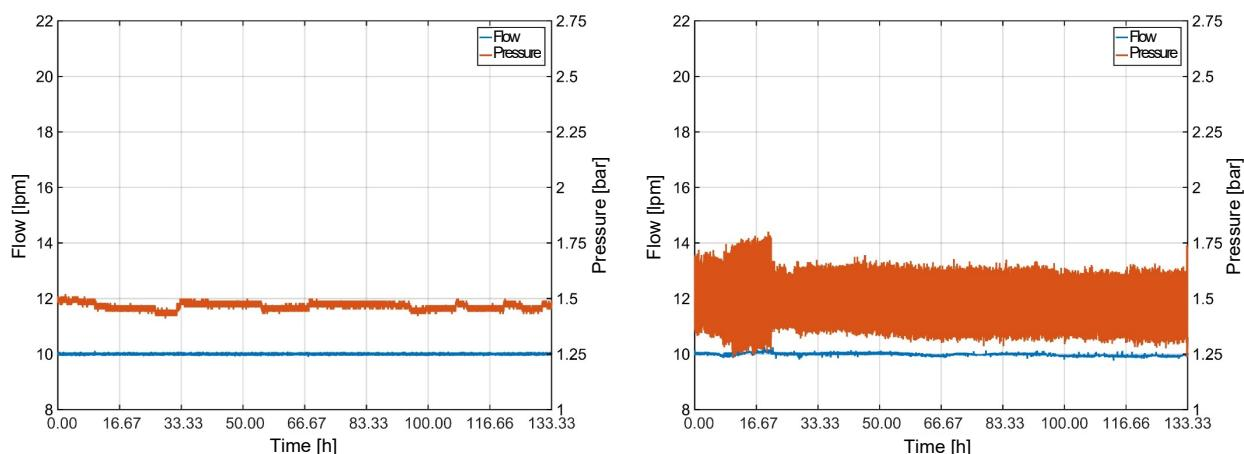
**Figure 3:** Representation of the online recorded pressure and flow rates during the experiment for the PuraLev® 600SU (P1.1 - left) and the 4-piston diaphragm pump (P1.2 - right) at a flow rate of 10 lpm and a pressure of 1.5 bar.
