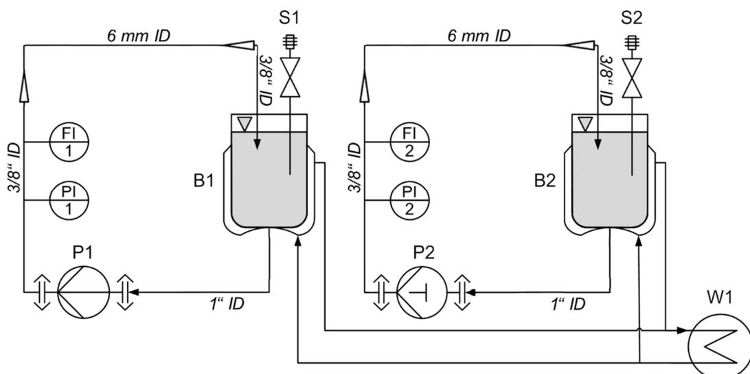
**Figure 1:** Schematic representation of the experimental setups for the Levitronix® PuraLev® 600SU (P1) and 4-piston diaphragm pump (P2). (S1) and (S2) sampling valve Clave Connector, (B1) and (B2) storage tank, (W1) thermostat, (FI1) and (FI2) flow sensor, (PI1) and (PI2) pressure sensor.
