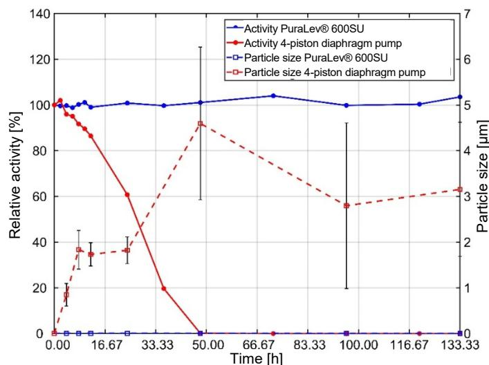
**Figure 2:** Results of the activity and dynamic light scattering measurements during pump experiments P1.1/P1.2 with the PuraLev® 600SU and the 4-piston diaphragm pump at a flow rate of 10 lpm and a pressure of 1.5 bar.
