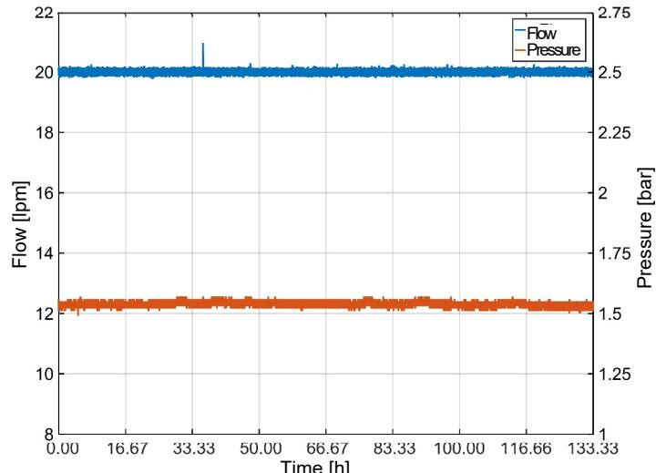
**Flow and pressure 4-piston diaphragm pump**
