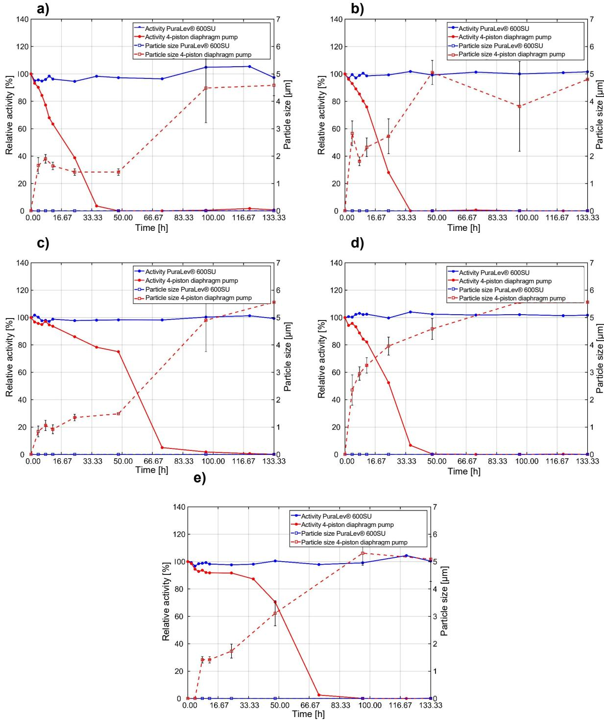
**Figure 5:** Results of the activity and dynamic light scattering measurements during the pumping tests with the PuraLev® 600SU and the 4-piston diaphragm pump at a flow rate of 10 lpm and 2.0 bar (P2.1/P2.2 - a), 10 lpm and 2.5 bar (P3.1/P3.2 - b), 20 lpm and 1.5 bar (P4.1/P4.2 - c), 20 lpm and 2.0 bar (P5.1/P5.2 - d) and 19 lpm and 2.5 bar (P6.1/P6.2 - e).
