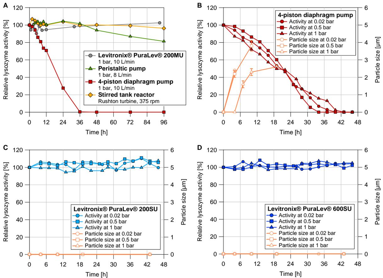
**Fig. 3:** Results of the activity and DLS measurements. (A) Preliminary experiment with the Levitronix® PuraLev® 200MU, the peristaltic pump, the 4-piston diaphragm pump and the stirred bioreactor. Main investigations with the (B) 4-piston diaphragm pump, (C) Levitronix® PuraLev® 200SU and (D) Levitronix® PuraLev® 600SU.
