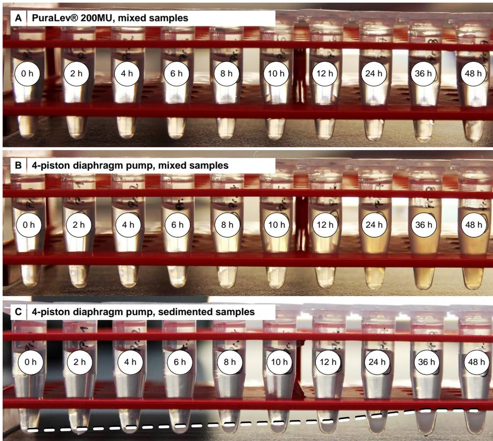
**Fig. 4:** Lysozyme solution turbidity over a 48 h pumping duration, for the PuraLev® 200MU (A) and the 4-piston diaphragm pump mixed samples (B) and settled samples (C).
