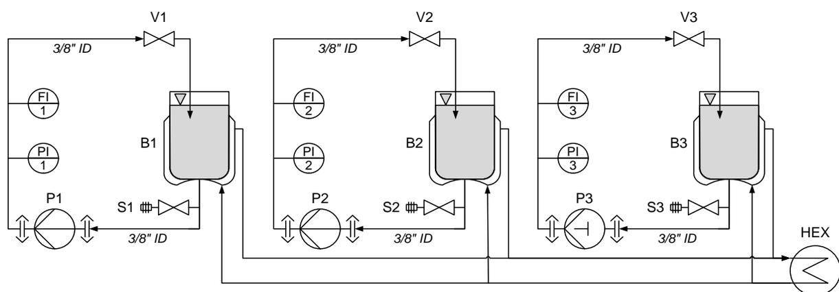
**Fig. 1:** Schematic of the experimental set-up for the evaluation of mechanical stress in PuraLev® 200SU (P1), PuraLev® 600SU (P2) and 4-piston diaphragm pumps (P3). (B1, B2, B3) Vessels, (FI1, FI2, FI3) flow sensors, (PI1, PI2, PI3) pressure sensors, (S1, S2, S3) sampling port, (HEX) thermostat. Hose clamps (V1, V2, V3) were installed if needed, depending on the operating pressure.
