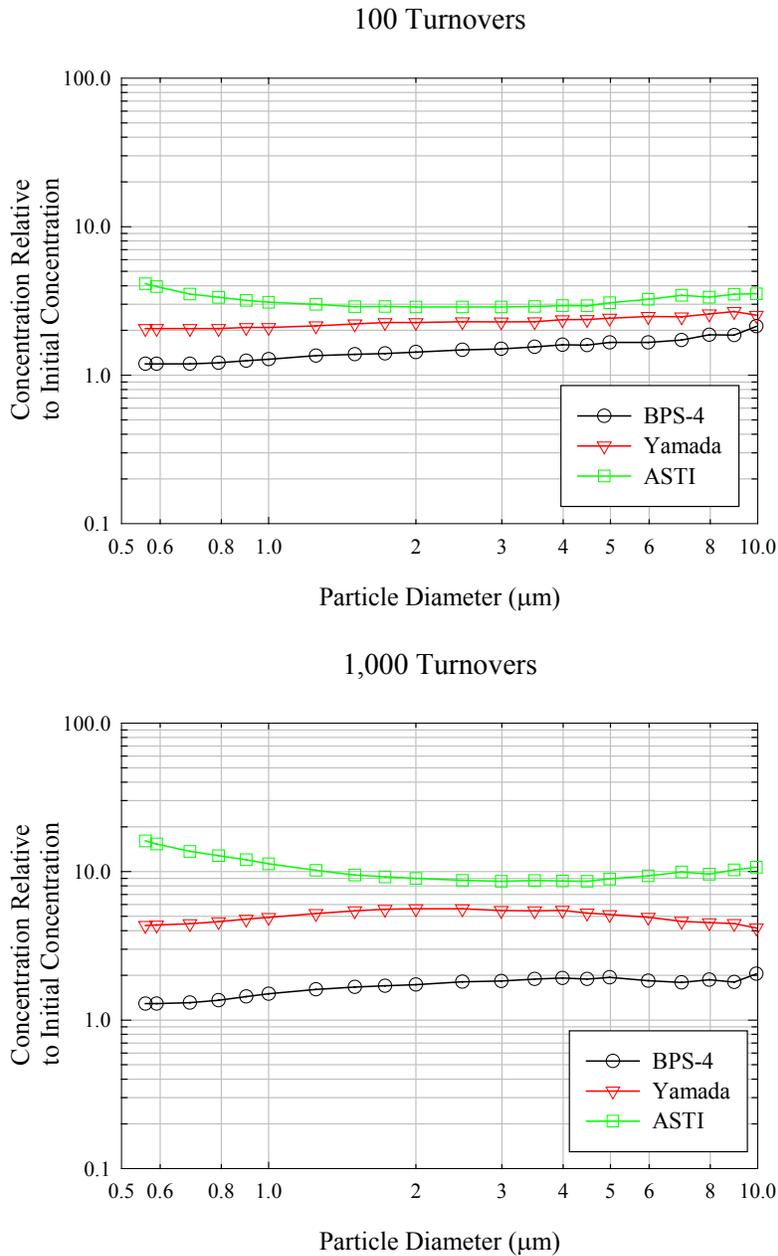
Table II shows a summary of the relative particle concentration changes during each test after approximately 100 and 1,000 turnovers for selected particle sizes.
