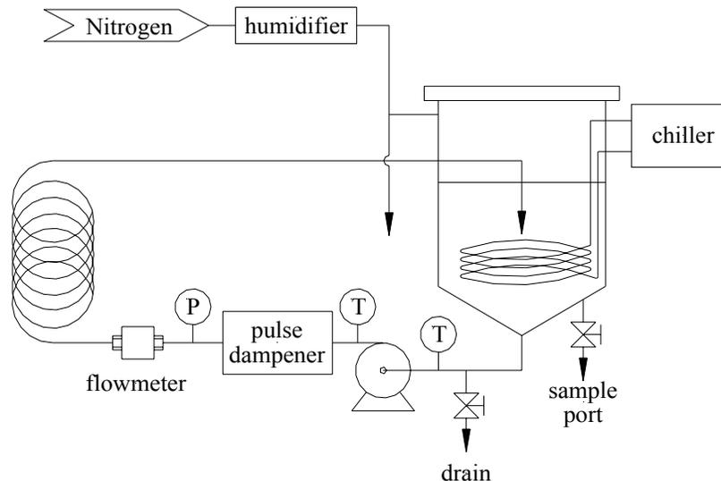
The tank holding the slurry was blanketed with nitrogen to prevent absorption of carbon dioxide from the air that can change the pH of the slurry. The nitrogen was humidified to prevent dehydration of the slurry. Shifts in the pH and dehydration can both result in particle agglomeration in the slurry. The relative humidity in the tank was > 90% throughout the test. A chiller and stainless steel coil were used to maintain the slurry at  $20 \pm 2^\circ\text{C}$  during the test.
