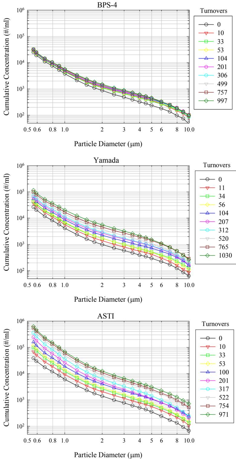
Small changes in the large particle tail of the slurry PSD were observed during the centrifugal pump test. Meanwhile, significant increases in large particle concentrations were observed during the Yamada and ASTI pump tests over a wide range of particle sizes.
