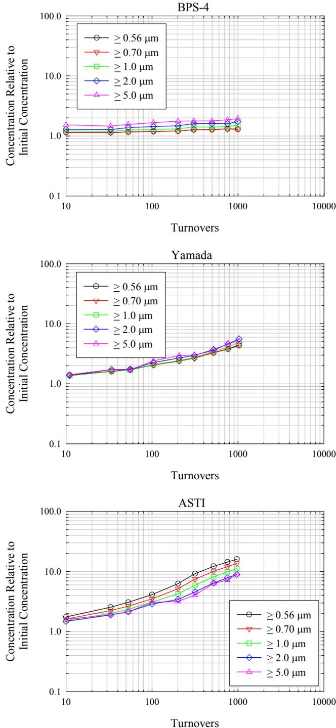
Figure 4 presents the particle concentration ratios during each pump test as a function of particle size after approximately 100 and 1,000 turnovers. These points were chosen since slurry is typically turned over on the order of 100 times prior to use, while 1,000 turnovers is believed to be a conservative upper estimate in most slurry delivery systems.
