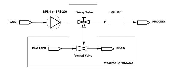
Figure 2: Flowplan of Bearingless Pump System for Low Flow Applications
