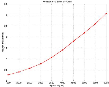
Figure 1: Process Flow in Relationship to Pump Speed in Water (Reducer: d = 0.2 mm, L = 70 mm)
